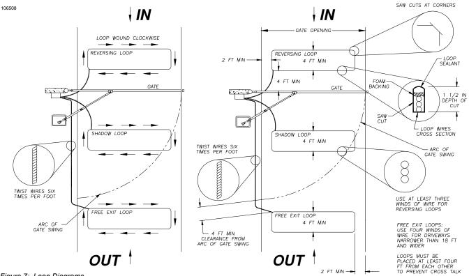
Figure 7: Loop Diagrams
